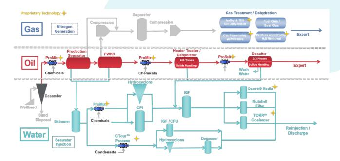
ProSep has a wide range of capabilities including crude dehydration and desalting, gas treatment and dehydration as well as a full lifecycle produced water treatment offering. ProSep Energy Services provides a diverse range of rental skids designed for the temporary treatment of a wide variety produced water streams.
