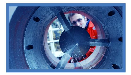
ProSep's mixing technologies differ from traditional inline mixing technologies as they utilize main stream momentum by reducing open flow area and increase flow velocity, resulting in a high mixing driving force.
